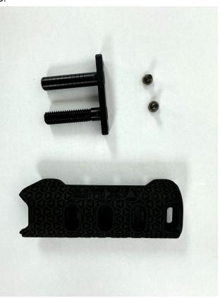
Next, Remove the two screws that attach the rods to the metal plate.
