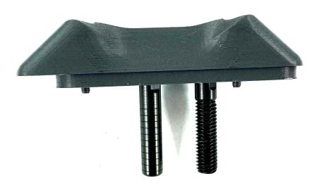
Keep the screws loose until you have found your desired position. Thread the assembly back into the chassis, and tighten the screws once you have found the proper position forward and back.
